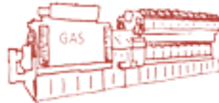
Gas - Up to 25 MVA
